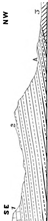
Section of north-west end of range east of Pakaraka Flat, showing the lower beds of coal-bearing strata near bridge at A. 1. Hydraulic limestone and firestone. 2. Greensands. 3. Old rock.
